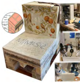
Prototype of historical wall with embedded sensors for pH and chlorides detection.
