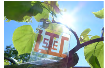
Prototype of Dye Sensitized Solar Cells (DSSC) for building integrated photovoltaics.
